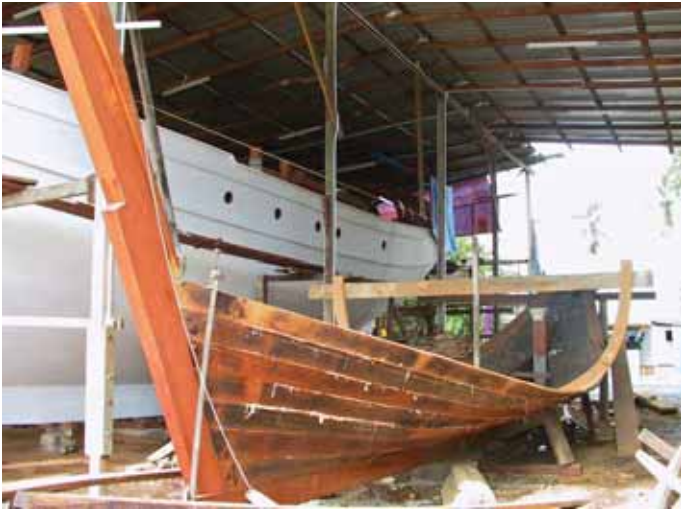
ABOVE: A fishing boat hull under construction LEFT: A traditional river boat takes shape
